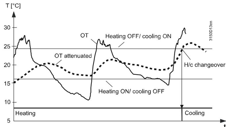
When value "Heating off/cooling on" is exceeded, the H/C changeover signal is changed to cooling. When "Heating on/cooling off" is below the set value, the H/C changeover signal is changed to heating. "Attenuation" can be set for the input signal.
