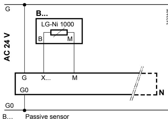
Example 2 Average temperature measurement with 2 passive sensors using LG-Ni1000 sensing elements.
