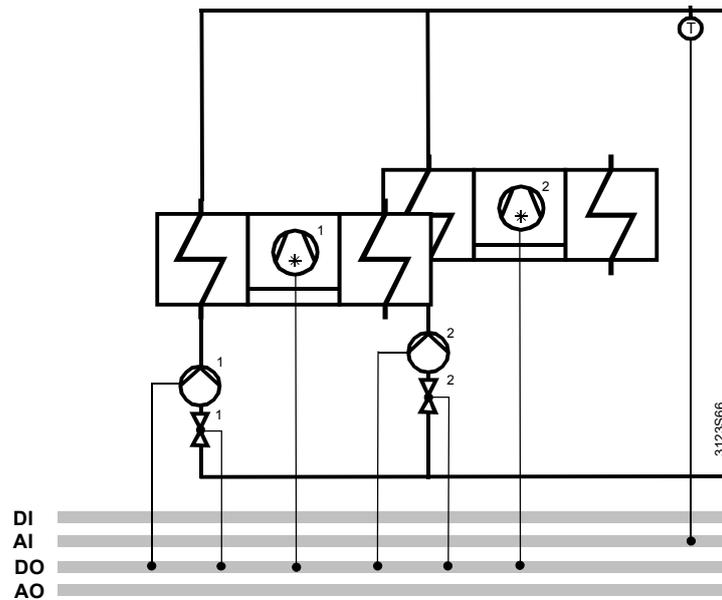
Configuration diagram: The precommand input e.g. is switched via signal "Plant on" (via Logic 1).
