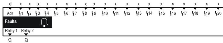
**Enabling** Enable the fault block by configuring fault inputs 1...20 or assigning a fault relay.
