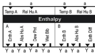
**Purpose** The function block calculates the following based on inputs temperature and relative humidity:
