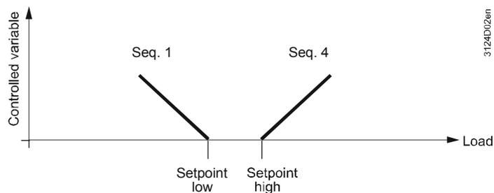
The "Setpoint low" (heating setpoint) is assigned to sequence 1. Its output signal acts reverse to the load (inputs variable).
