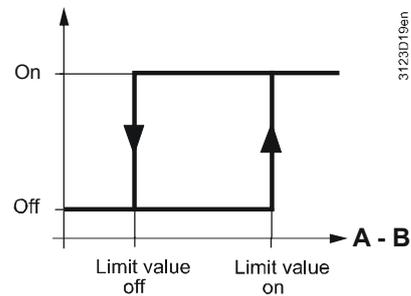
Min. switch-on and switch-off times can be set for the output signal of the comparator along with a switch-on and switch-off delay.
