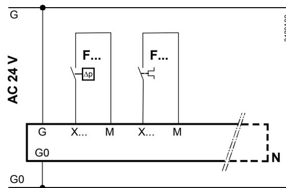
F... Detector with potential-free switching contact.
