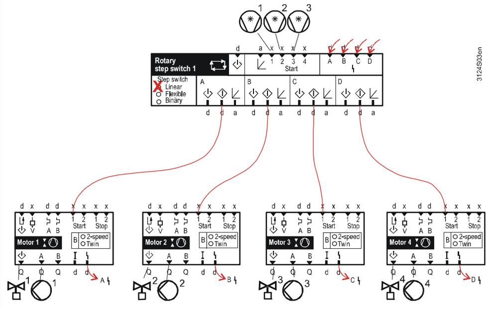
\* The start conditions of the rotary step switch are configured as per the refrigeration machine releases.
