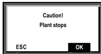
Press OK again to stop the plant (application). All outputs are set to a defined OFF state and the display shows the "Commissioning" menu.
