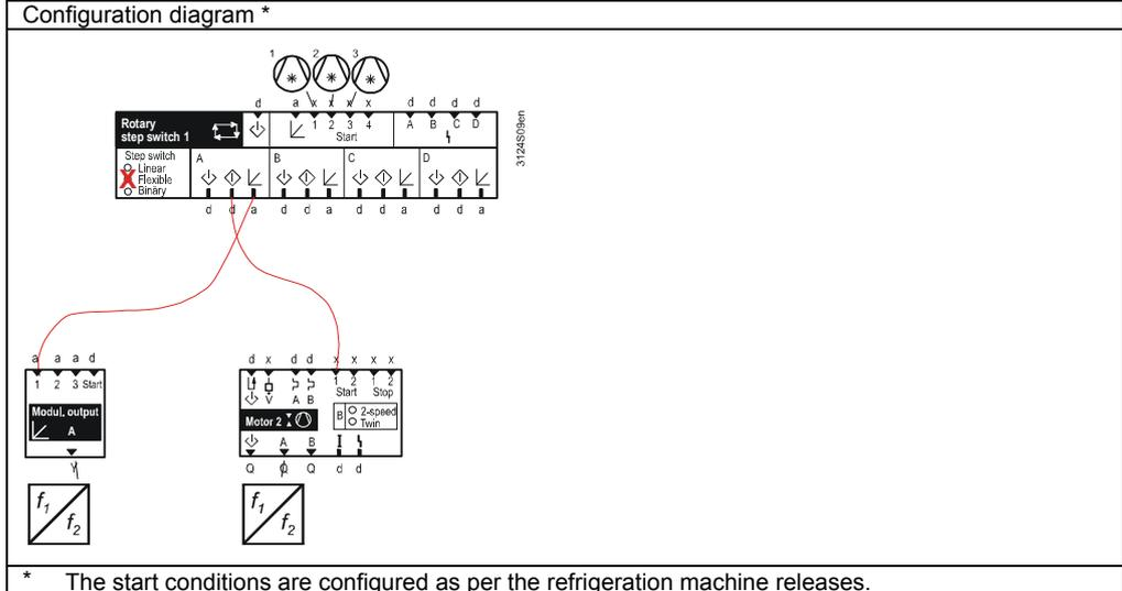
\* The start conditions are configured as per the refrigeration machine releases.
