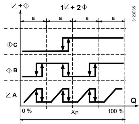
The following overview shows configurations for using the binary rotary step switch.
